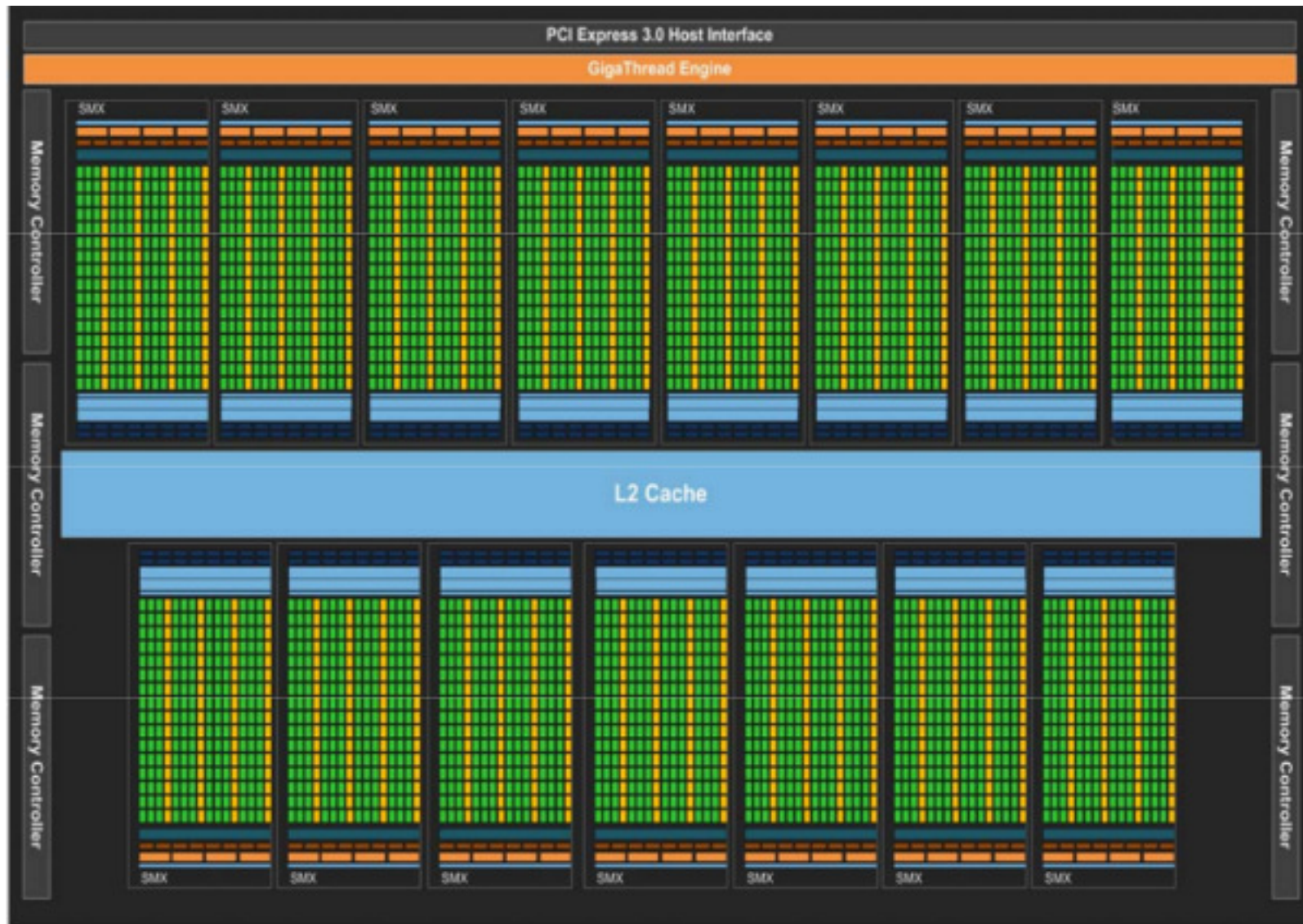
Nvidia's Kepler architecture as of 2012 (192 single-precision cores / 15 SMX)
